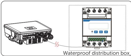
Figure 15-28 Connecting inverter to meter
