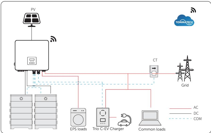
Figure 15-5 Trio C-EV Charger wiring diagram
