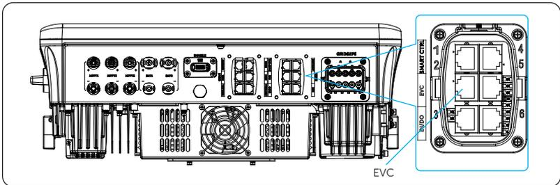
Figure 15-6 Connection terminal for Trio C-EV Charger
