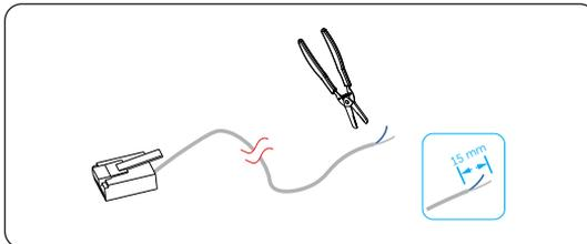
Figure 15-23 Stripping communication cable for meter
