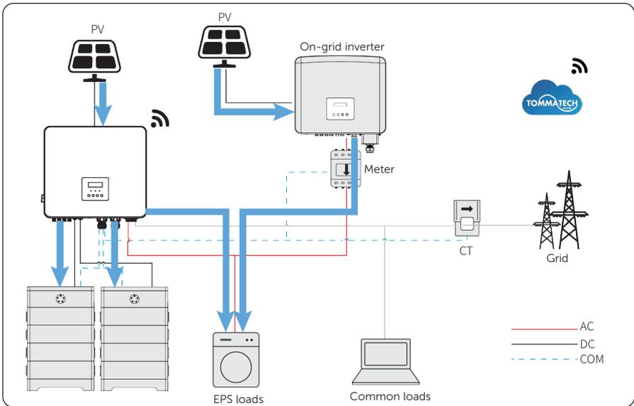
Figure 15-13 Power flowing when grid off
