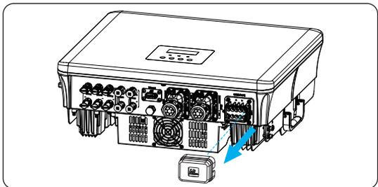
Figure 8-19 Removing the cap
