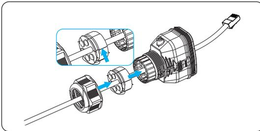
Figure 8-39 Threading the cable with the RJ45 terminal
