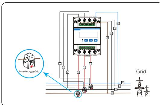
Figure 15-26 Connecting CT-connected meter to the grid
