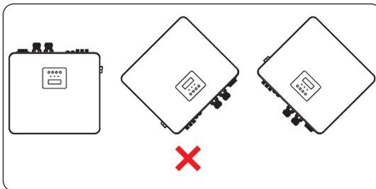
Figure 7-2 Incorrect installation
