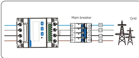
Figure 15-22 Connecting direct-connected meter to the grid
