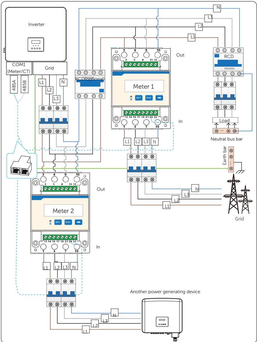
Figure 15-30 Connection diagram of two direct-connected meters
