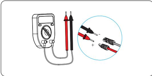
Figure 8-27 Measuring the voltage of PV connectors
