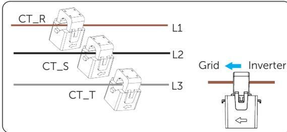
Figure 15-19 Clipping CTs to grid cables
