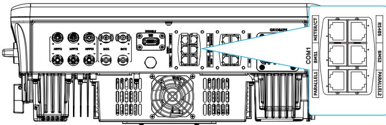
Figure 8-36 Overall layout of terminal COM 1
