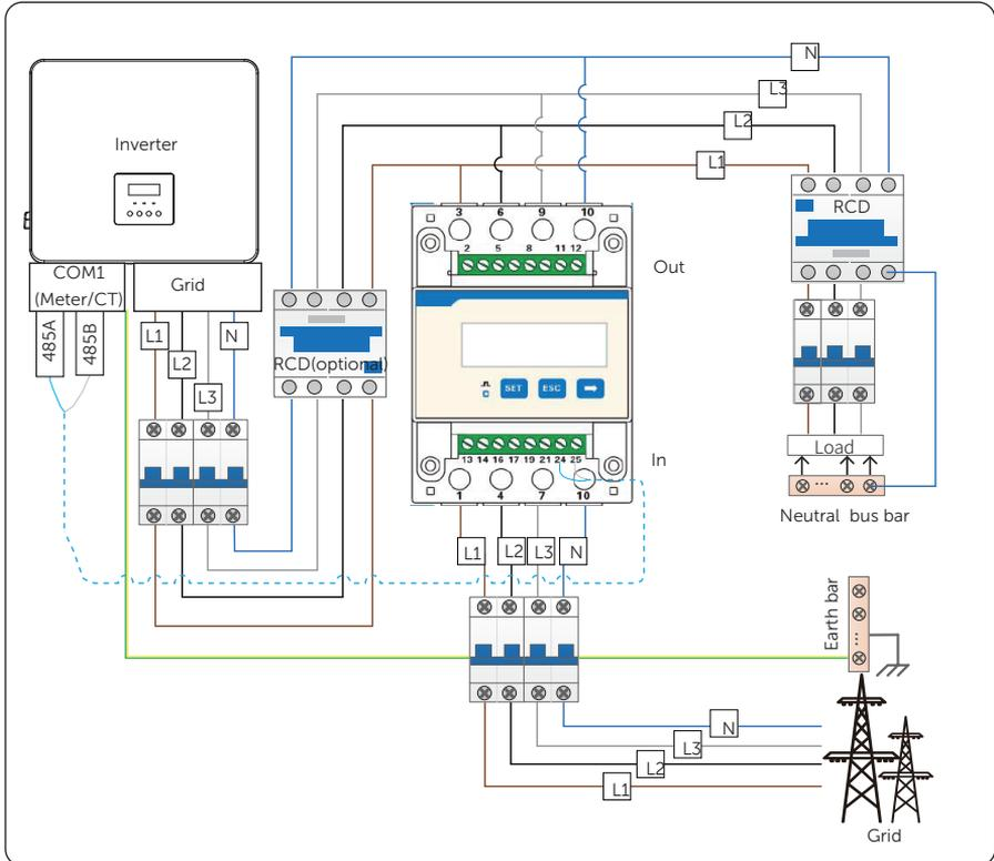
Figure 15-21 System wiring with direct-connected meter
