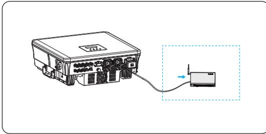
Figure 8-53 Connecting to Smart Controller
