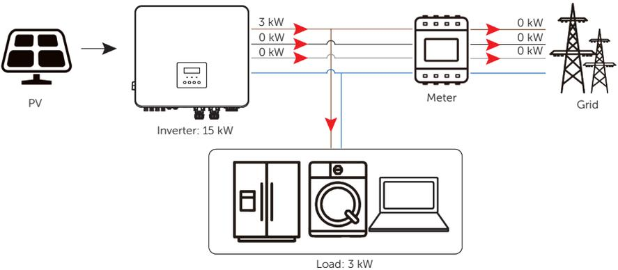
Figure 2-14 Zero export control with **Phase Unbalance** enabled
