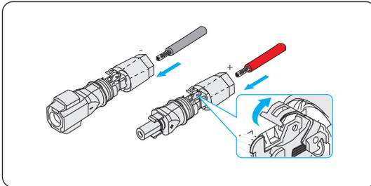
Figure 8-31 Inserting the cable into the battery connector
