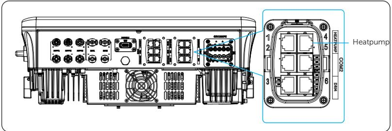
Figure 15-4 Connection terminal for Heatpump Controller
