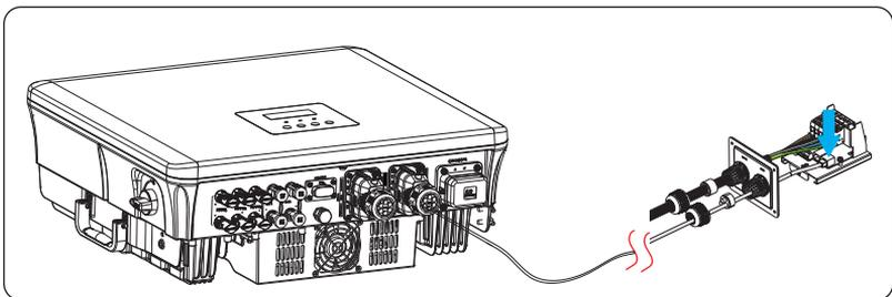
Figure 15-7 Connecting to Trio C-EV Charger
