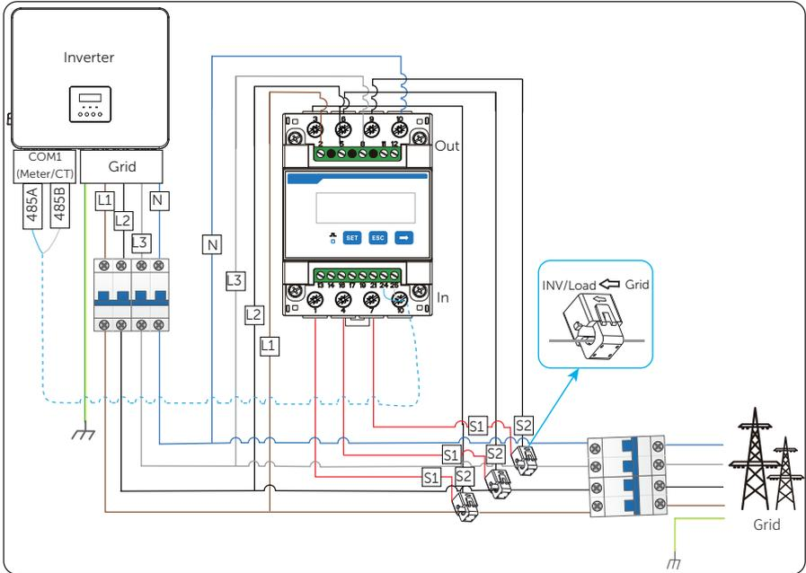
Figure 15-25 System wiring with TommaTech CT-connected meter
