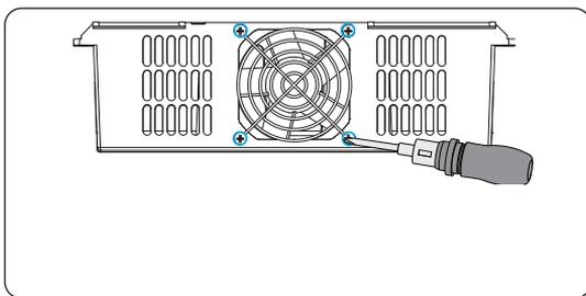
**Step 4:** Replace with a new fan (pay attention to the installation direction of the fan) and fasten the screws for the fan.
