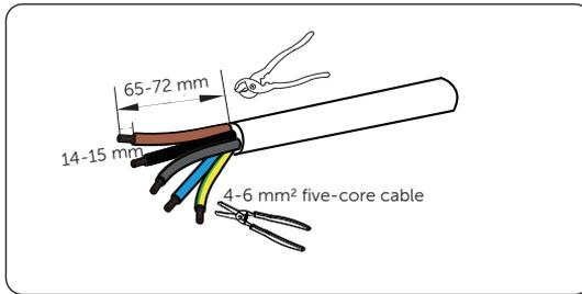
Figure 8-9 Stripping the Grid and EPS cables
