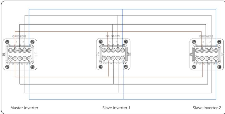
Figure 15-16 Power cable wiring
