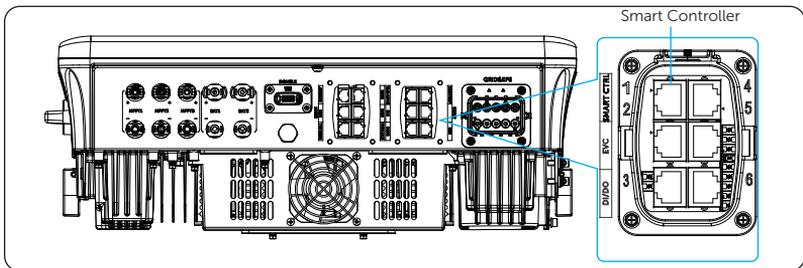
Figure 15-9 Connection terminal for Smart Controller
