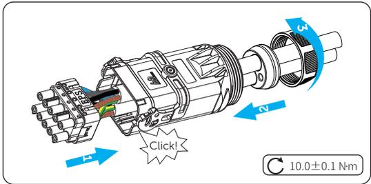
Figure 8-18 Assembling the AC connector
