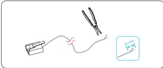
Figure 15-27 Stripping communication cable for meter
