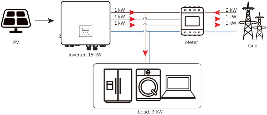
Figure 2-13 Zero export control with **Phase Unbalance** disabled
