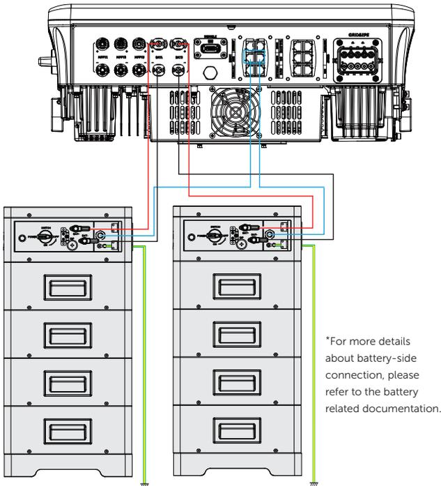
Figure 8-45 BMS connection diagram
