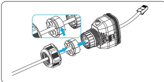
Figure 8-49 Threading the cable with the RJ45 terminal
