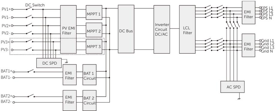
Figure 2-5 Circuit diagram of Trio Hybrid Pro Series inverter
