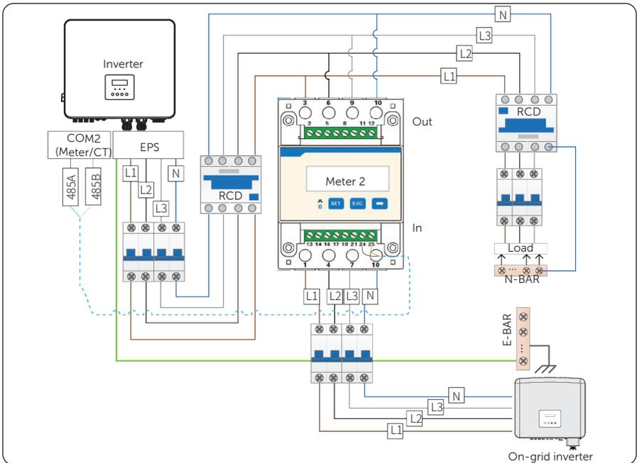
Figure 15-14 Connection diagram of Meter on EPS terminal
