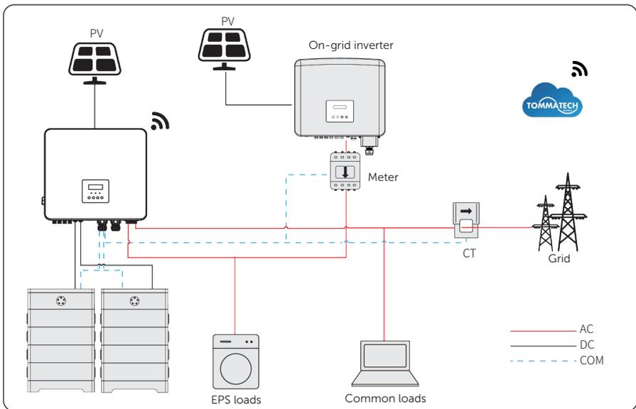
Figure 15-11 Micro-grid wiring connection
