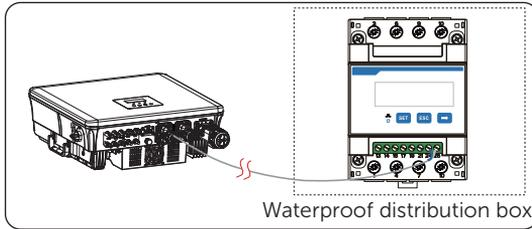
Figure 15-24 Connecting inverter to TommaTech meter
