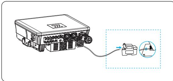
Figure 15-20 Connecting the inverter to the CT
