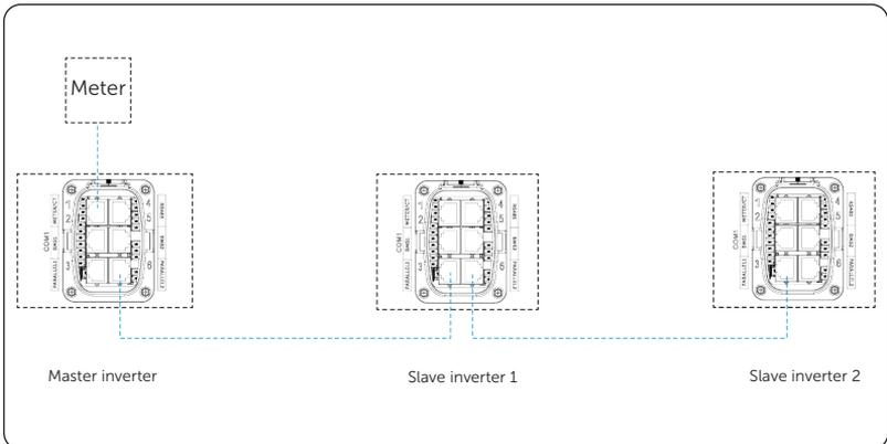
Figure 15-17 Communication wiring
