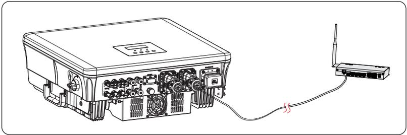
Figure 15-10 Connecting to Smart Controller
