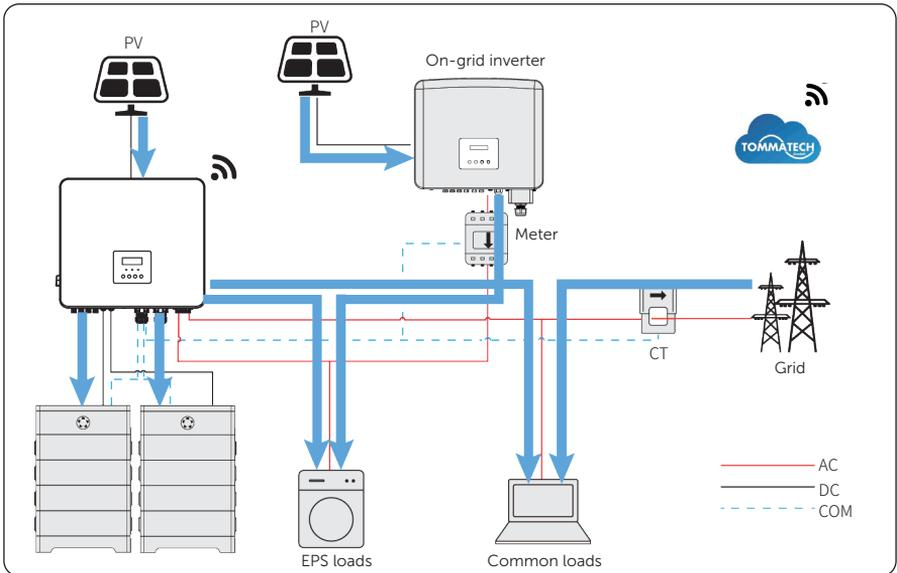
Figure 15-12 Power flowing when grid on and PV sufficient
