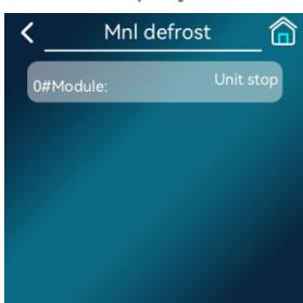
If you need to defrost manually, first select on the corresponding module and the manual defrost approval box will pop up. Please select **ü** to start the defrosting.
