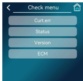
If the heat pump is in fault or error mode, press the "Curt.err" option to view the error.
