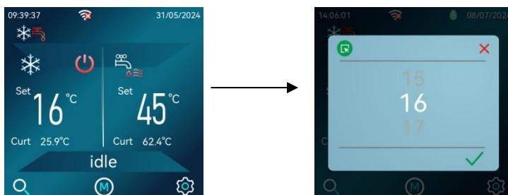
Select the target value by sliding and then press **✓** to modify the set temperature value.
