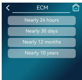
The operation of this wire controller to check the Power, Capacity and COP(EER) in any time period is the same. However, we will show how to get the data of the last 30 days as an example:
