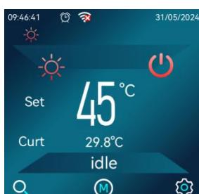
The timer icon will not be shown on the main interface when the timer is invalid or inactive..
