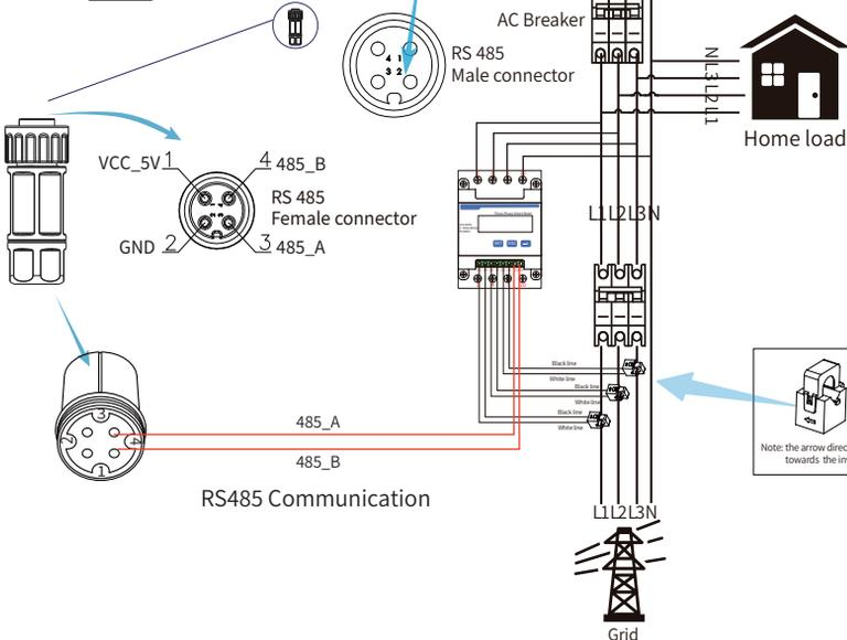
Pic 7.14 Connection diagram of CHINT meter
