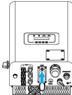
Pic 5.10 Datalogger installation diagram
