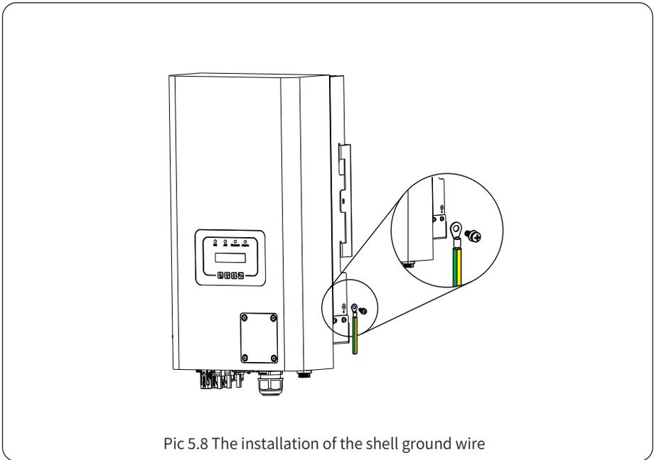
Pic 5.8 The installation of the shell ground wire
