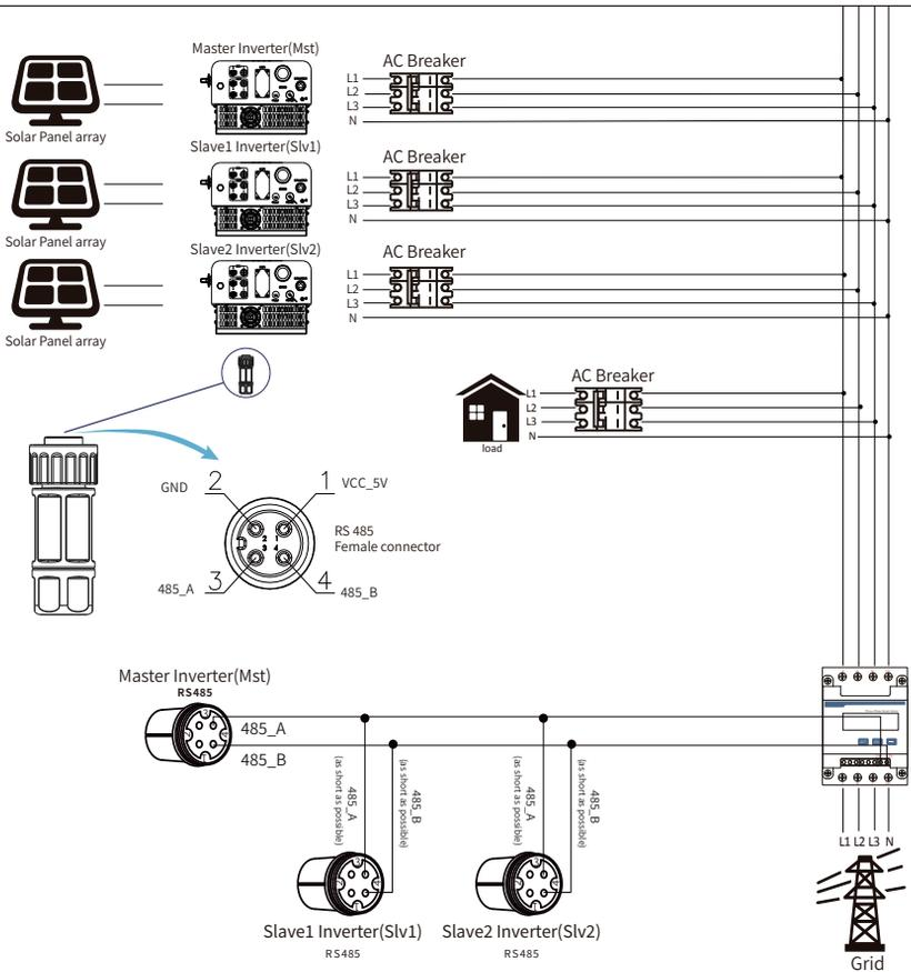
Pic 7.27 CHINT Connection diagram(The pass-through table)
