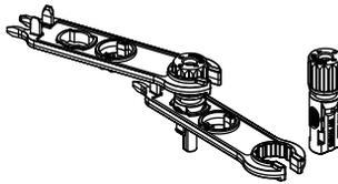
Pic 5.5 connector with cap nut screwed on
