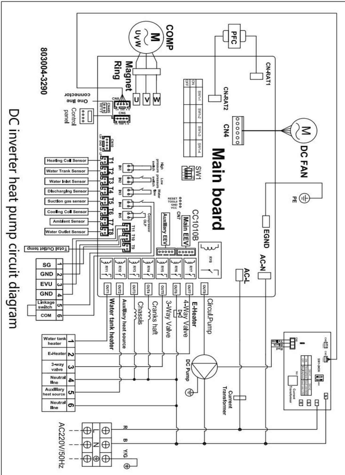
DC inverter heat pump circuit diagram
