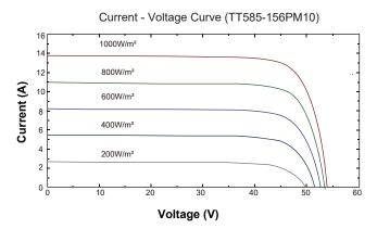
\*Note 1: The specifications are obtained under the standard test conditions: 1000W/m2 solar irradiance, 1.5 Air Mass and cell temperature of 25°C. Measurement uncertainty for all panels is 6%. The actual transactions will be subject to the contracts. These parameters are for reference only and it is not a part of the contracts. The specifications are subject to change without prior notice.
