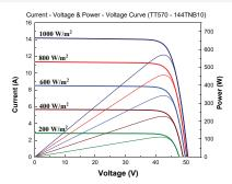
\* The specifications are obtained under the standard test conditions: 1000W/m2 solar irradiance, 1.5 Air Mass and cell temperature of 25°C. Measurement uncertainty for all panels is 6%. The actual transactions will be subject to the contracts. These parameters are for reference only and it is not a part of the contracts. The specifications are subject to change without prior notice.
