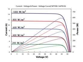
\* The specifications are obtained under the standard test conditions: 1000W/m2 solar irradiance, 1.5 Air Mass and cell temperature of 25°C. Measurement uncertainty for all panels is 3%. The actual transactions will be subject to the contracts. These parameters are for reference only and it is not a part of the contracts. The technical specifications in this document may vary. For more information, refer to the "Installation Manual".
