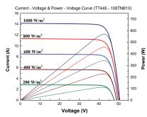
\*Note 1: The specifications are obtained under the standard test conditions: 1000W/m2 solar irradiance, 1.5 Air Mass and cell temperature of 25°C. Measurement uncertainty for all panels is 6%. The actual transactions will be subject to the contracts. These parameters are for reference only and it is not a part of the contracts. The specifications are subject to change without prior notice.
