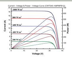
The specifications are obtained under the standard test conditions: 1000W/m2 solar irradiance, 1.5 Air Mass and cell temperature of 25°C. Measurement uncertainty for all panels is 3%. The actual transactions will be subject
