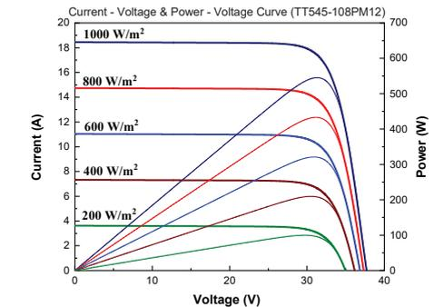
\* The specifications are obtained under the standard test conditions: 1000W/m<sup>2</sup> solar irradiance, 1.5 Air Mass and cell temperature of 25°C. Measurement uncertainty for all panels is 6%. The actual transactions will be subject to the contracts. These parameters are for reference only and it is not a part of the contracts. The technical specifications in this document may vary. For more information, refer to the "Installation Manual".
