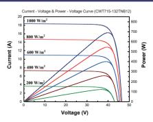
The specifications are obtained under the standard test conditions: 1000W/m2 solar irradiance, 1.5 Air Mass and cell temperature of 25°C. Measurement uncertainty for all panels is 3%. The actual transactions will be subject to the contracts. These parameters are for reference only and it is not a part of the contracts. The technical specifications in this document may vary. For more information, refer to the "Installation Manual".
